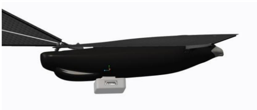
To charge MetaBird, simply insert MetaBird's connectors into the charging slot of the adapter. Then connect the cable to your smartphone charger or to a USB socket of your computer.
