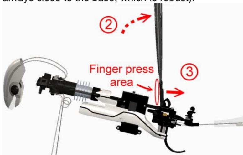
2 – Once in position, rotate the tail up to a vertical position, then 3 – **slide your forefinger down** at maximum to press it backward into the final position.
