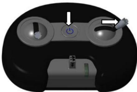
Step1- Push the direction Stick to the far right and keep it while pushing the power button
