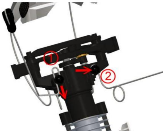
1 - Slide the “hook” at the end of the leg below the screw head (the screws come already assembled on the frame).
