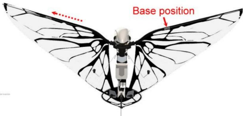
Each wing is equipped with a ballast. Its base position is nearest to the body. It can slide toward the end to create a ballast differential between the 2 wings.
