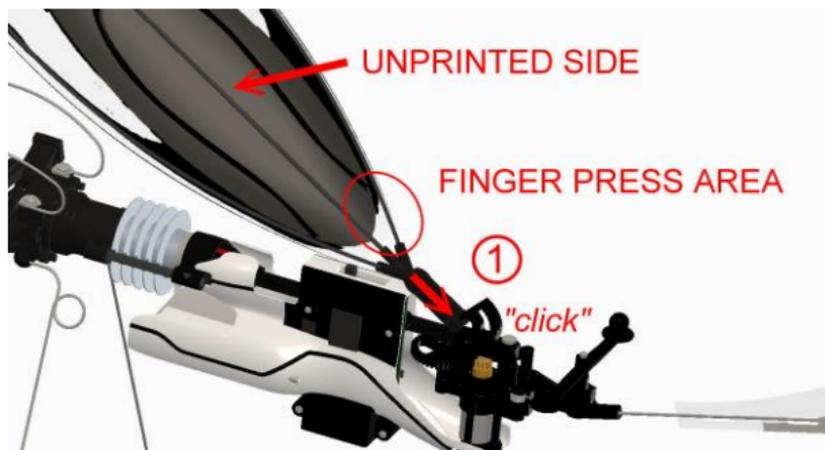
1 - Snap the tail end into its hole by pushing following the arrow direction until you feel a “click”. Mind your fingers position as shown on the picture. (hold the tail always close to the base, which is robust).
